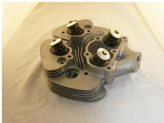
The valve springs are made from today's very best materials: super clean Silicon Chromium Vanadium Nickel alloy steel, which is especially intended for the manufacture of valve springs and other springs requiring high fatigue properties and good relaxation properties. The springs are made in the UK to the original BSA specification for the BSA 500cc DBD and 350 cc DB motors (BSA part nos. 65-2495 inner and 65-2494 outer).
