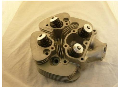
The conversion uses premium quality valve springs made from the best materials and alloy valve spring retainers made from aerospace certificated bar stock.
